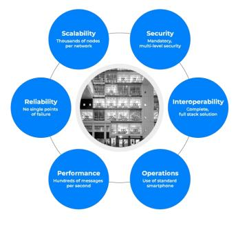
NOTE- Source [https://www.bluetooth.com/] Figure 3-14: Features of Bluetooth Mesh
